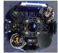
the AGV with dual 2-DOF wheels
